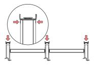
Adjust horizontal profile to desired position. Tighten socket screws with 3mm hex key to secure position.
