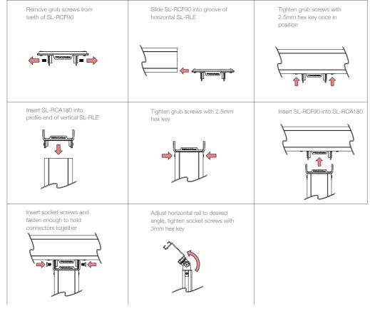
Creating and decorating aluminium framework has never been faster or more flexible. With only one profile required and adaptable connectors, the Stratlock Rail System is a foolproof way to create a consistent substrate for the perfect panel finish.. For further information or technical support contact: info@fastmount.com
