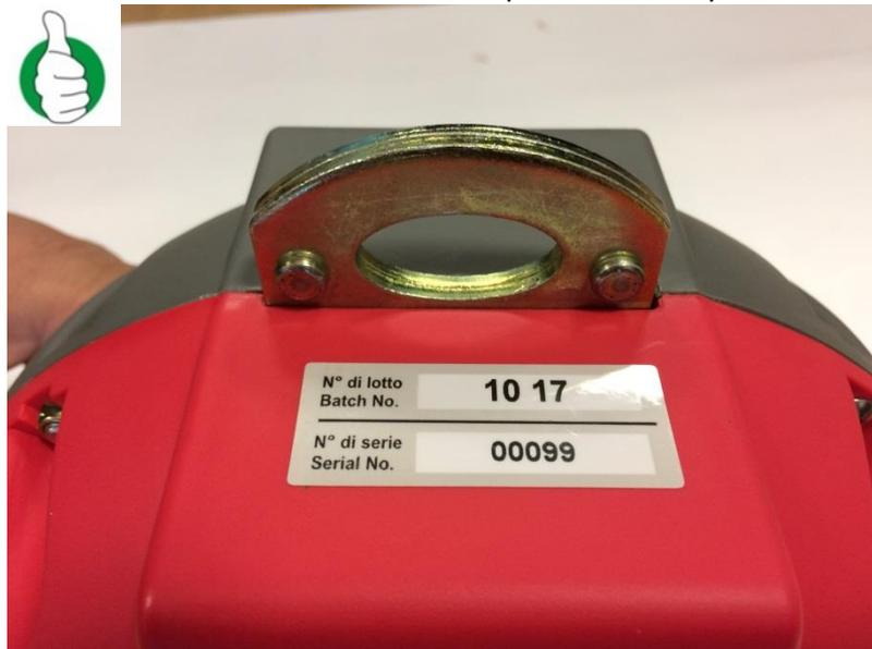
**Example No.2:** substituted rivets. The device has been already inspected and opened in the past by a centre that is authorised by the manufacturer.
