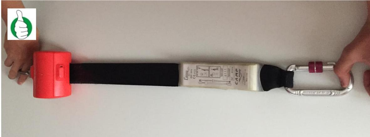
**Example No.1:** Check the strap connection on the drum.
