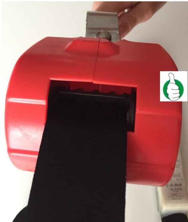
**Example No.2:** Verify the swivel device movement and inspect the ring (corrosion, cracks, deformations).
