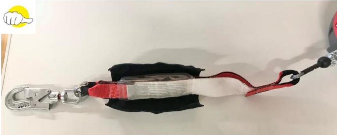
Check/verify any cuts, bulges, stiffening, damages, wear, exposure to heat and chemicals of the absorber webbing.
