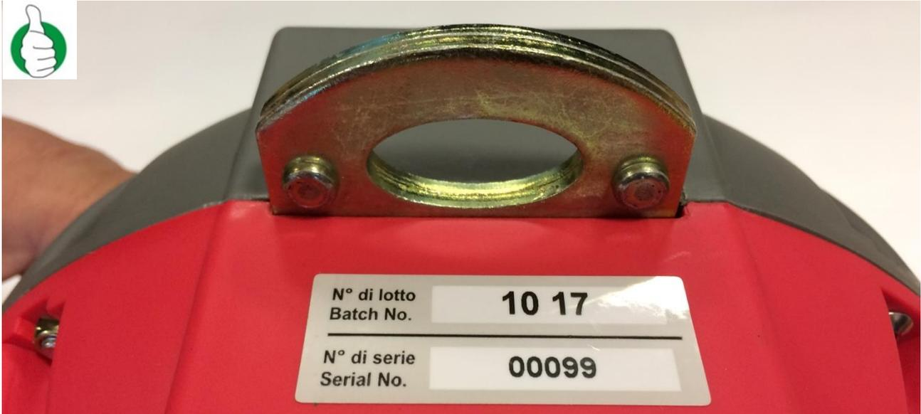
**Examples:** Thoroughly verify the wire entry/exit bushing. Should nicks with a depth exceeding 1 mm be present, withdraw the device from service and send it to a revision centre authorised by the manufacturer.
