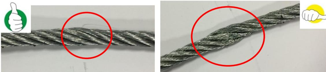
**Example No. 2:** Frayed metal wire: it is necessary to withdraw it from service and send it to a revision centre authorised by the manufacturer.
