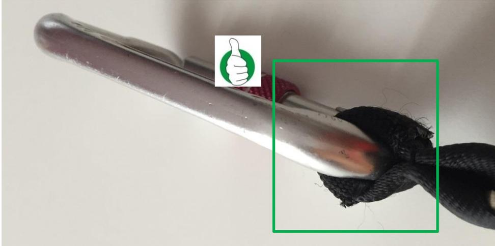
**Example no. 7:** Thoroughly verify the conditions of the shock absorber. If you notice marks of complete or partial opening of the shock absorber (even if only 5 mm-long), the device was employed in a fall arrest and has to be **WITHDRAWN FROM SERVICE**.
