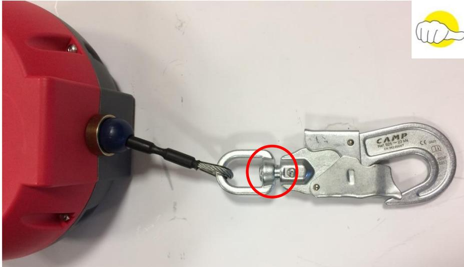
**Example No.3:** Connector with a ring, which cannot be seen. A repair is needed.
