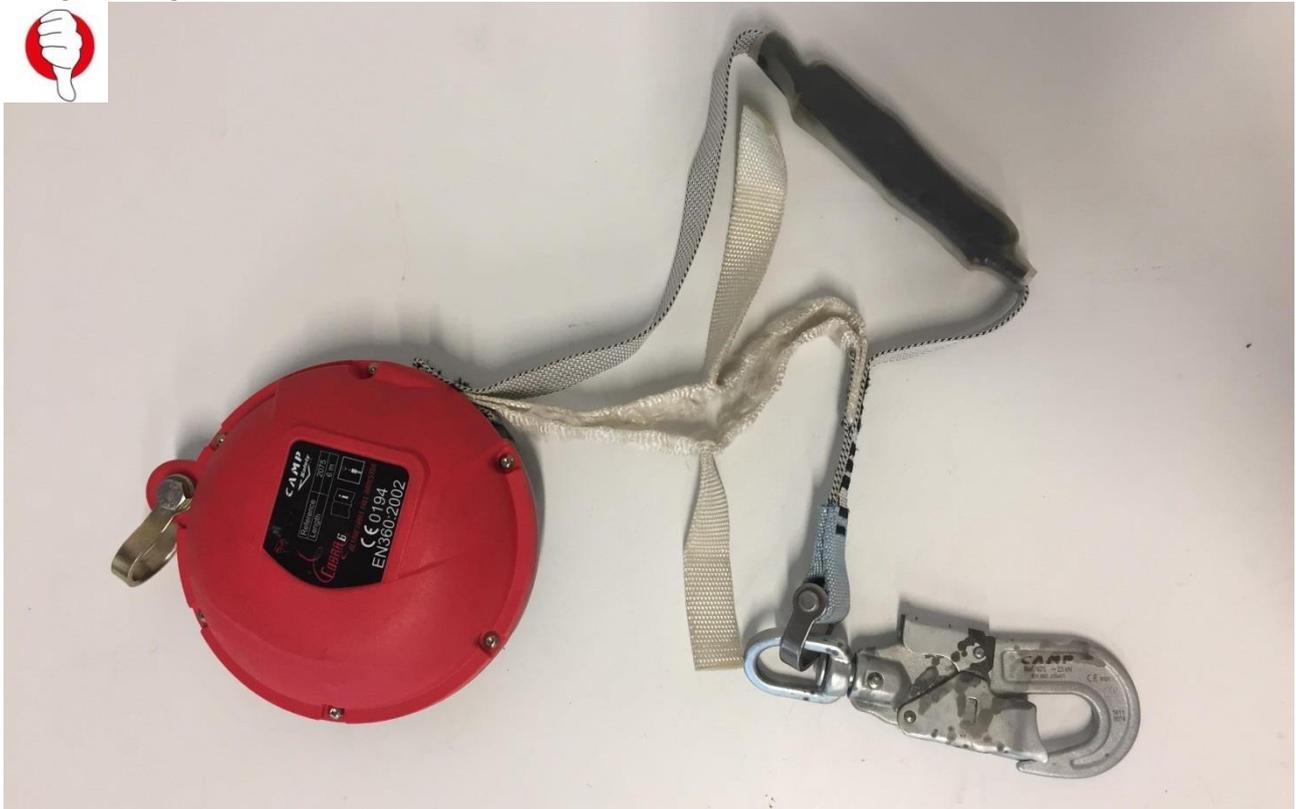
**Warning:** The inspection is **NEGATIVE** even with a partial opening of the shock absorber.
