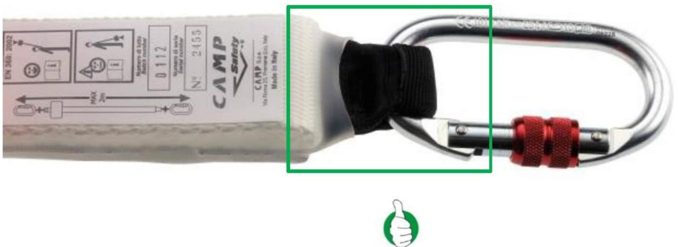
**Example No.6:** Thoroughly analyse the contact surfaces between the textile parts, paying great attention to any wear mark, cuts, burns and ripping. Pay special attention when analysing the stitch points.
