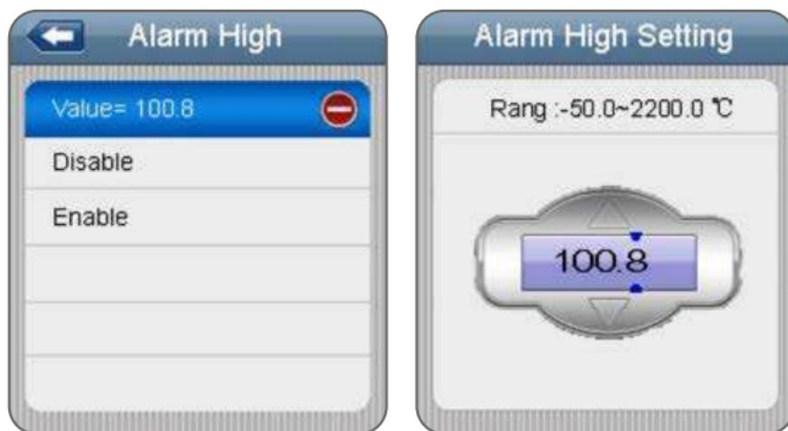
Press the ENTER button on the first row and use the UP and DOWN button to adjust the value. Press the ENTER button to confirm, press the ESC button to esc and save.
