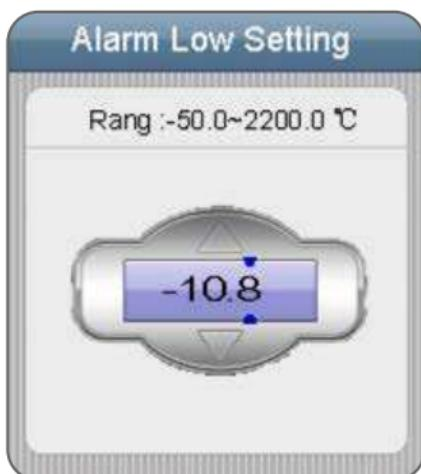
Press the ENTER button on the first row and use the UP and DOWN button to adjust value. Press the ENTER button to confirm, press the ESC button to esc and save.
