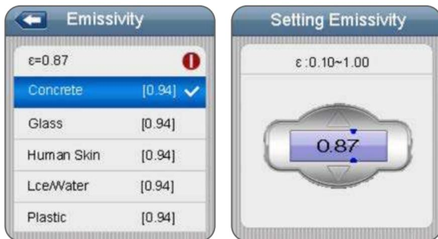
ON the first Item, press the ENTER button to adjust emissivity, press the UP and DOWN button to adjust the value, then press the ENTER button to confirm. Press the UP and DOWN button to select the emissivities of the materials, press the ESC button to esc and save.
