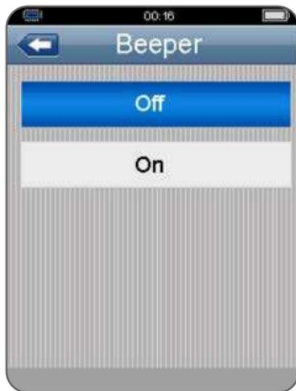
Press the UP and DOWN button to select the beeper status, press ESC button to esc and save the select the beeper status.
