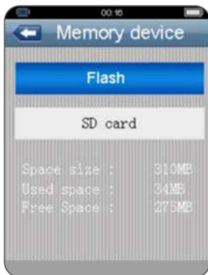
Press the UP and DOWN button to select the Memory device, press the ENTER button to enter. The internal memory or the memory card can be selected.
