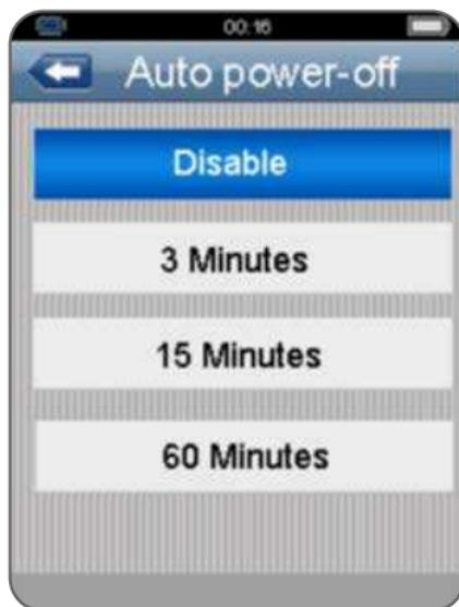
Press the UP and DOWN button to select the auto power off time or never auto power off, press the ESC button to esc and save.
