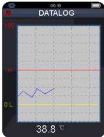
Press the trigger once to start the datalogger measurements.
